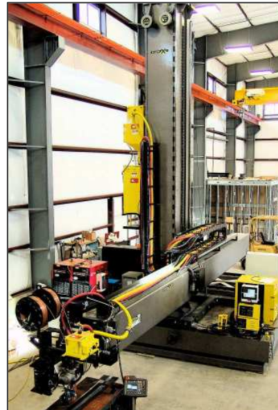
CBM-HD-7x4.5 with XM controlled Lincoln Tandem SAW Babcock Wilcox Canada
